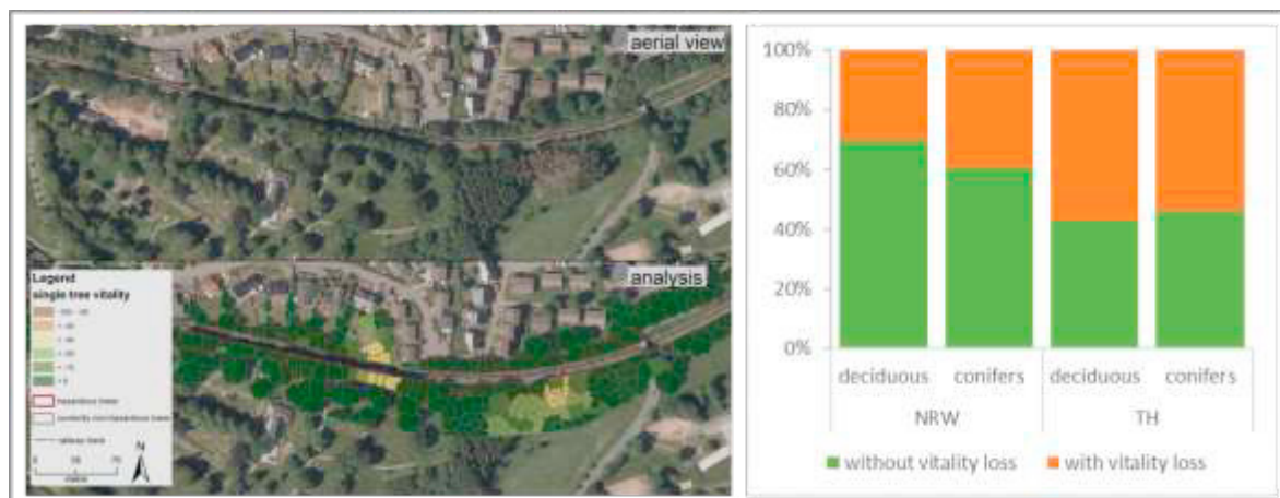
Fig. 4. An example of monitoring tree vitality along the railway network of Northrhine-Westphalia (left), and percentage of trees with and without vitality losses in 2020 in the close vicinity of the railway network in the federal states Northrhine-Westphalia (NRW) and Thuringia (TH), classified into deciduous trees and conifers (right). The vitality loss for 2020 is calculated as the difference to a reference year (2017 for NRW, 2018 for TH).
